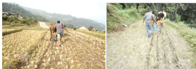
Fig. 3 Animal drawn Single row zero till planter Fig. 4 Animal drawn two rows zero till planter
