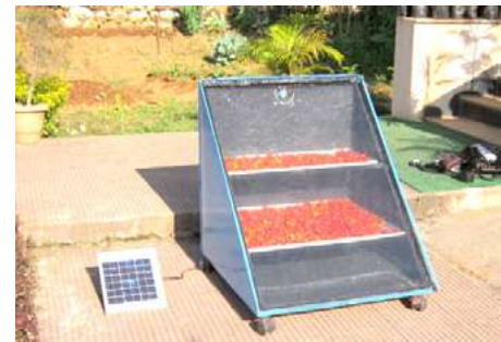
Fig. 1 Portable solar PV powered force convection solar dryer loaded with chilly
