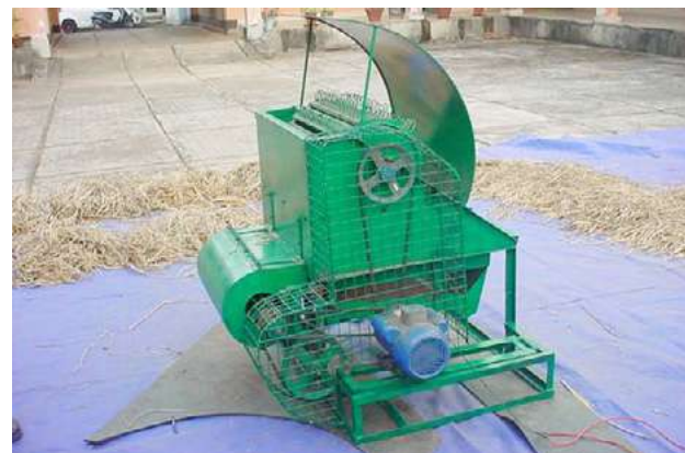
Fig. 3 Light weight powered paddy thresher cum cleaner
